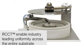
The developer can perform both puddle and spray-based processes.
