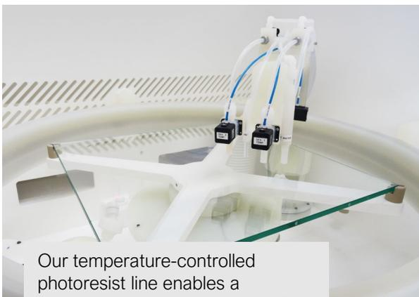
Our temperature-controlled photoresist line enables a repeatable temperature level of the photoresist, the developer or chemicals substrate-to-substrate at point of dispense.
