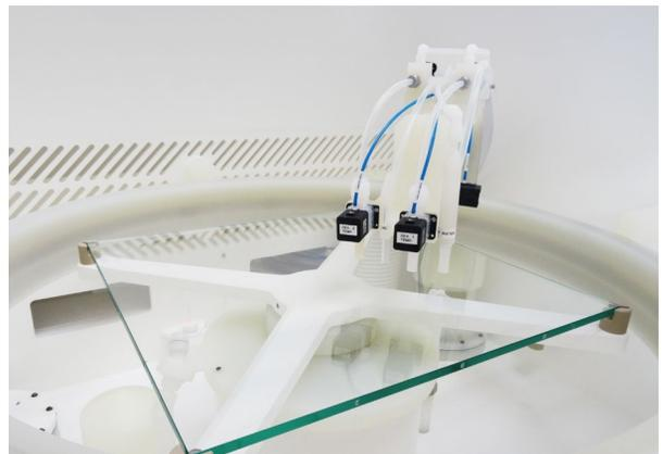
Our temperature-controlled photoresist line enables a repeatable temperature level of the photoresist, the developer or chemicals substrate-to-substrate at point of dispense.
